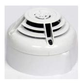
The NRX-TDIFF heat sensor is a battery operated RF device designed for use with the NRXI-GATE radio gateway. It contains a wireless transceiver and runs on a NOTIFIER intelligent fire system (using a compatible proprietary communication protocol). The NRX-TDIFF provides 58°C rate-of-rise (10°C/minute) temperature sensing (A1R).
