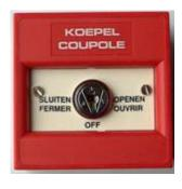
Key switch as external priority control with open, close and neutral position. The key switch contains electronics to connect this three position switch with only two, polarity independent wires, to the Sahep panel. The connection is supervised with a built in end of line resistor. Maximum one SAHEP-PRIOR can be added on a Sahep panel.
