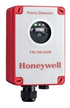
Analyses the flame flicker frequency to improve false alarm rejection, the dual sensing methodology enable the effectively detection of a wide range of hydrocarbon and non-hydrocarbon fires. It offers also a good resistance against direct and reflected sunlight and artificial light, arcs and electric discharge.
