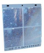
The BEAM-LRK kit contains 3 reflectors (200mm x 230mm). In combination with the short range reflector supplied with the beam, the 4 reflectors mounted in square form one big reflector surface which extends the beam range over 70m, up to a maximum distance of 100m.
