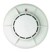
The ECO1002 multi-criteria detector uses a state of the art optical chamber and a class A1R thermal element combined with a microprocessor, running sophisticated algorithms to provide quick and accurate detection of fires.
