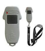
The remote control for Testifire is required for situations where the IR test beam of Testifire that triggers or stops a test is not broken by a physical presence. Typical situations are the sampling ports of aspirating detection systems or detectors with 'virtual chambers'. The Testifire 25 is then used to initiate the test procedure.
