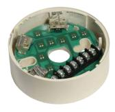
Standard base with heater, compatible with the NFXI series. Rises the temperature of the detector to avoid condensation in the detection room.
