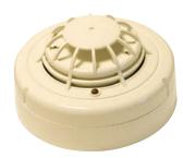
The FD-851TE thermal detector incorporates the latest in thermal element technology, the detector provides efficient and accurate detection of fires, especially in environments such as boiler houses or kitchens where smoke detectors are inappropriate due to the high level of airborne contamination.
