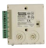
The M701 control module provides a monitored single output circuit for use with polarised loads (sounder circuit) which requires a suitable power source (7VDC - 30VDC) for the connected load. Alternatively the same device may be placed in to an unsupervised mode which can then be used to control any switched load up to 2A @ 30VDC.
