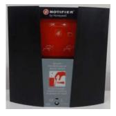
This slave panel can be connected to the SAHEP-4N and provides 8A with battery backup. This slave panel can be installed close to the smoke vent which leads to short high current wiring for the motors. On this slave panel a 70°C temperature sensor can be added providing a failsafe opening system. Even when the connection with the master panel fails, the slave panel will open the smoke vent at 70°C.
