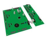
Provides 16 LEDs or relays outputs. Up to 9 expansion boards can be daisy chained. Requires 020-741 IDR-CM Mimic main board. For use with "local zones".
