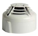
The NRX-SMT3 radio sensor is a battery operated RF device designed for use with the NRXI-GATE radio gateway. It contains a wireless transceiver and runs on a NOTIFIER intelligent fire system (using a compatible proprietary communication protocol). It is a multi-criteria smoke and heat detector (58°C Rate-of-Rise). An infrared sensor adds further detection ability and increased immunity to false alarms. The sensor plugs into the B501RF wireless sensor base (not included).
