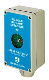
The IR flame detector model RIV-601P/F is an electronic optical fire detecting device which responds immediately to the thermal infrared radiation emitted by fire and is turned to the flickering frequency of the flame to ignore sun and lamp light.
