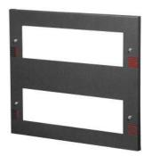
Includes moulding, hinges for user interface door, push clip fasteners and printer slot covering label. Finished in RAL7021. Moulding adds 21 mm to overall depth of back box. (To cover 256 zone display module 020-612).
