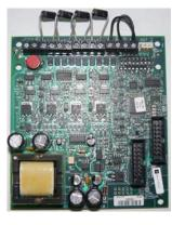
Provides 4 monitored circuits with provision for external PSU and 2 digital inputs.
