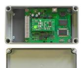
This interface has two RS232 communication ports to connect the NF30/50 and NF3000 NOTIFIER fire panel to a Pager system using the Standard Espa444 protocol. Both RS232 communication are constantly monitored. Communication based on TPP11, it doesn't support addresses above 99 and Sub address.
