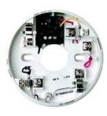
Interface for 24V system that requires an external contact. The detector stays in alarm until the removing of its supply voltage. A break-off tab allows the base to be connected to fire control panels. This tab should be broken when there is little current flow or no current limiting resistor such as when used as a 24V stand-alone system.
