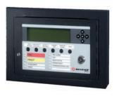
Active repeater, displays all alarm and fault messages on the LCD. Includes function pushbuttons as mute buzzer, accept, evacuate, resound sounders and reset. 240 x 64 Graphic LCD and status indication leds. Includes text insert label kit (NL, FR).
