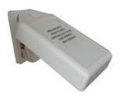
The SAHEP-RD rain detector functions with a capacitive sensor. So rain is detected in a capacitive way. In a capacitive rain sensor no external PCB traces are visible. These traces are sensitive for oxidation. This rain detector is compatible with the WRD1. A mounting bracket in included.
