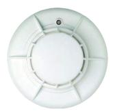
The ECO1004T detector uses a state of the art class BS and A1R thermal element combined with a microprocessor, running sophisticated algorithms to provide quick and accurate detection of fires. The detection incorporates a static element and is suitable where ambient conditions normally inhibit rapid changes in temperature, eg kitchens.
