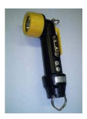
The PTL-611 portable test lamp is a plastic explosion-proof shock-proof and antistatic torch lamp with high intensity light which is modulated at a frequency of 23Hz so as to be used for external testing of RIV-601/F IR flame detectors, as an alternative to the internal test feature built-in inside these detectors.
