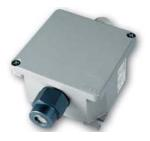
Gas detectors series SMART3 NC have been designed to offer cost effective products with Hi-Tech professional features for car parks and non-classified areas. Available only for Methane, LPG, Petrol Vapours, CO, NO2 and CO2, these detectors employ a professional catalytic sensor for flammable gas detection, an electrochemical cell for CO and an infrared sensor for the CO2 detection.
