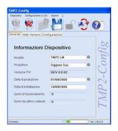
Special software for TMP2 heat detectors maintenance and configuration. Data Log capability, Trends, Calibration report, Stand-Alone calibration station. Complete of USB/RS485 connection cable.
