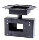
Ceiling pendant mount for use with F5000, F50/100, prism and 5000-005 universal bracket. Includes universal mounting plate. Does not include universal mounting brackets or 5000 detectors. Ceiling pendant mount comes with a 1" x 12" long threaded nipple. Contractor shall provide other nipple lengths as required.
