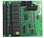
8 relay outputs which are configurable as N/O or N/C by jumper links (1A @ 30VDC). Link setting allows 4 function presets to be configured for all 8 relays.
