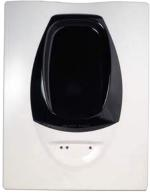
The 6500R and 6500RS detectors are combined transmitter/receiver units, which can be directly connected to a conventional zone and require a resetable 24VDC power supply. The Infra-Red transmitter generates a beam of light towards a high
