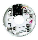
Interface for 12V systems that latches the detector into alarm. The detector can only be reset by removing its supply voltage. The base can be used with 4 wire security systems that have a reset facility.
