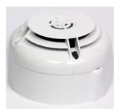
The NRX-OPT is a battery operated RF optical device designed for use with the NRXI-GATE radio gateway. It contains a wireless transceiver and runs on a NOTIFIER intelligent fire system (using a compatible proprietary communication protocol). The RF sensor plugs into the B501RF wireless sensor base (not included).
