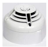
The NRX-TFIX58 heat sensor is a battery operated RF device designed for use with the NRXI-GATE radio gateway. It contains a wireless transceiver and runs on a NOTIFIER intelligent fire system (using a compatible proprietary communication protocol). The NRX-TFIX58 provides 58°C temperature sensing (A1S). The sensor plugs into the B501RF wireless sensor base (not included).
